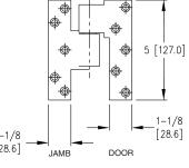
Technical Note: On labeled door NFPA 80 requires one intermediate pivot per door height up to 90" (2286)mm and two intermediate pivots for doors from 90"(2286)mm to 120" (3048)mm
